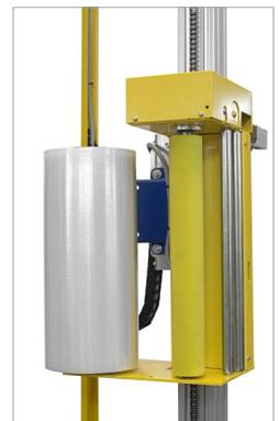
In addition, with larger volumes, different sizes and types of products, the user has a choice of the **CA6** carriage with a **1 motor powered film roll brake** (fixed pre-stretch of 150, 200 or 250%) or the **CA7** carriage with two motor-driven **power pre-stretch**. Delivering between 120 and 350%. (1 meter becomes 4,5 meters of film).
